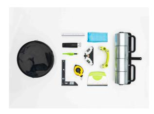
Determine the installation direction of the Moduleo® flooring. Calculate how the partition of the planks or tiles will be across the width of the room/area and mark a 100% straight line on the floor with help of a chalk line/laser line, normally in parallel with the longest straight wall.
